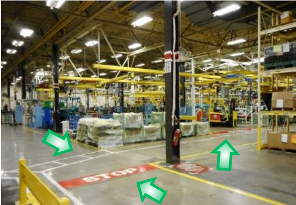
Floor stops added, crosswalk and aisle painted.
