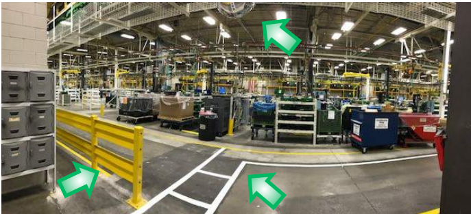
Rail extended due to blind corner, crosswalk painted, aisle extended, globe mirror added.
